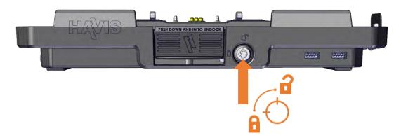
2) Unlatch Rear Hooks by a pushing down on Release Handle, then b pushing in until a click can be heard.
